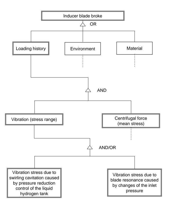
Fig.4 Fault tree diagram for loading history, environment and material
