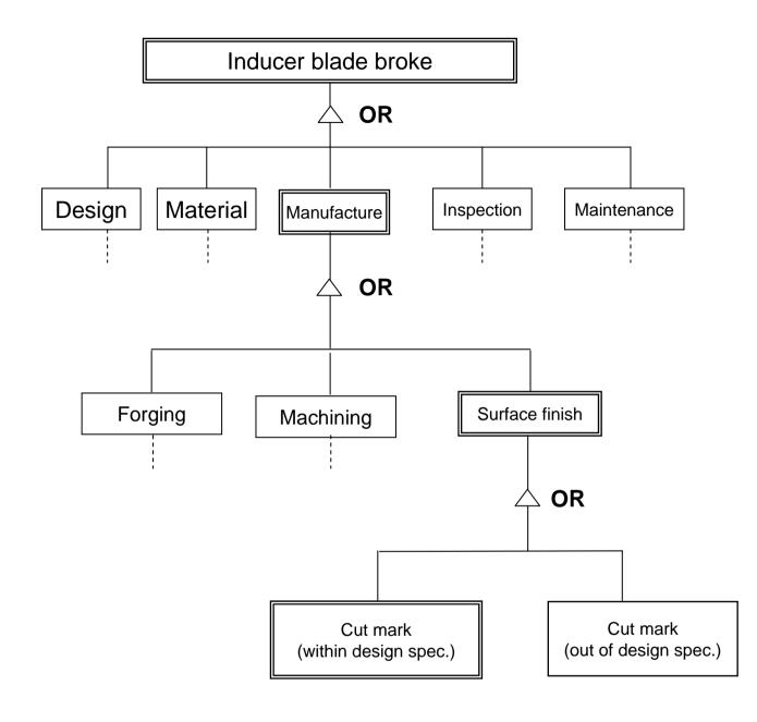
Fig.3 Fault tree diagram for design and manufacturing errors
