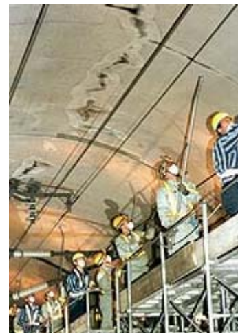
Figure 4. Hammering test (Source: Chugoku newspaper)
