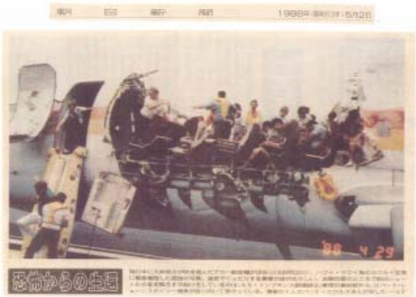
Fig. 1 B-737 Made an Emergency Landing with Large-scale Peeling of Fuselage.
