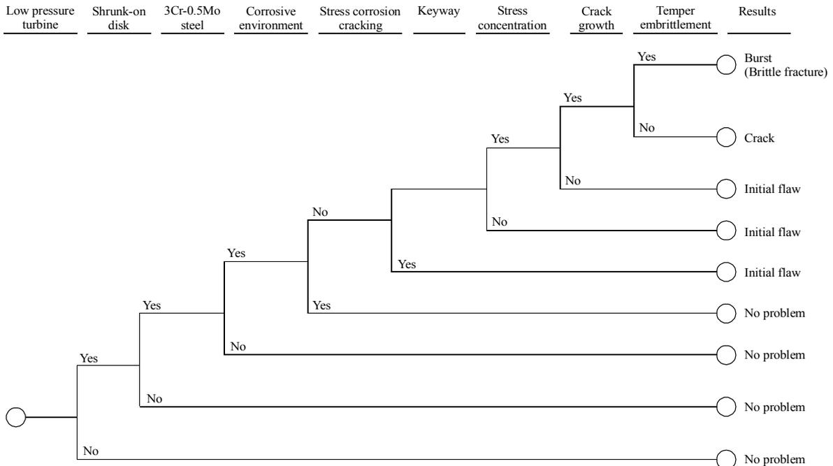
Fig. 6 Event tree diagram for the low-pressure steam turbine rotor burst attributed to stress concentration in a shrunk-on disc keyway and the low toughness of a disc material.
