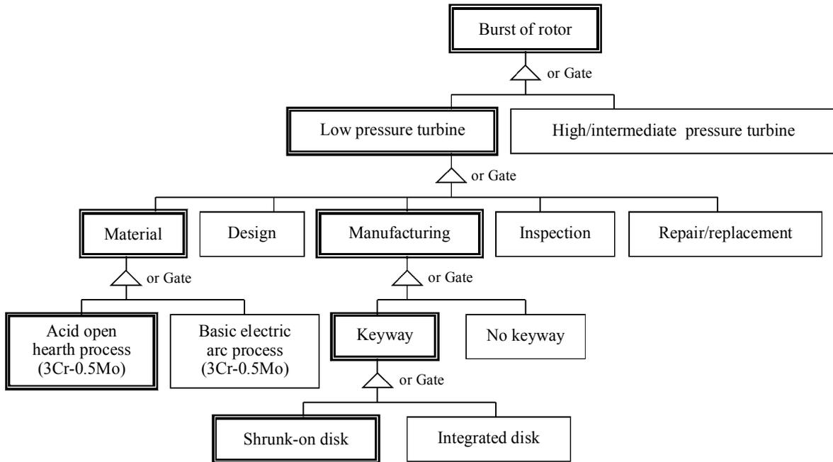
Fig. 5 Fault tree diagram for design and manufacturing errors.
