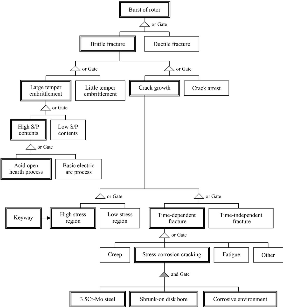
Fig. 4 Fault tree diagram for mode, mechanism and process of fracture.
