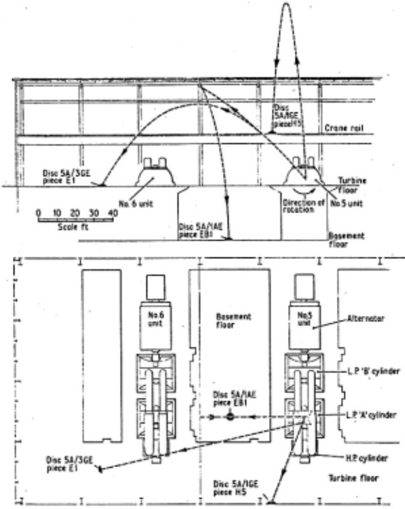
Fig. 3 Flying-off paths of three large disc fragments.
