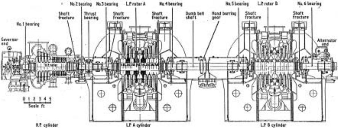
Fig. 1 Overview of the burst TVA Gallatin No.2 IP-LP turbine rotor.
