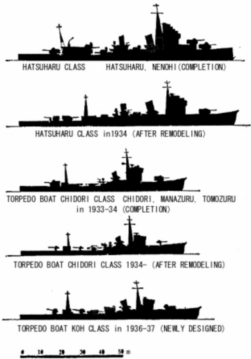
Fig.4 Change of the Destroyers and Torpedo Boats' shape. (Before and After Remodeling)
